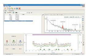
spectrum view of stored spectra and actual analysis results of isotope identification. User comments can be added to the measured data by using the built-in active notepad. All information is easily exported and then used in external software packages like Google Earth to plot GPS information.
